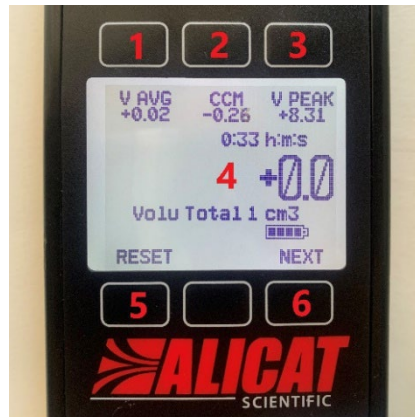
Figure 5. Totalized flow data
